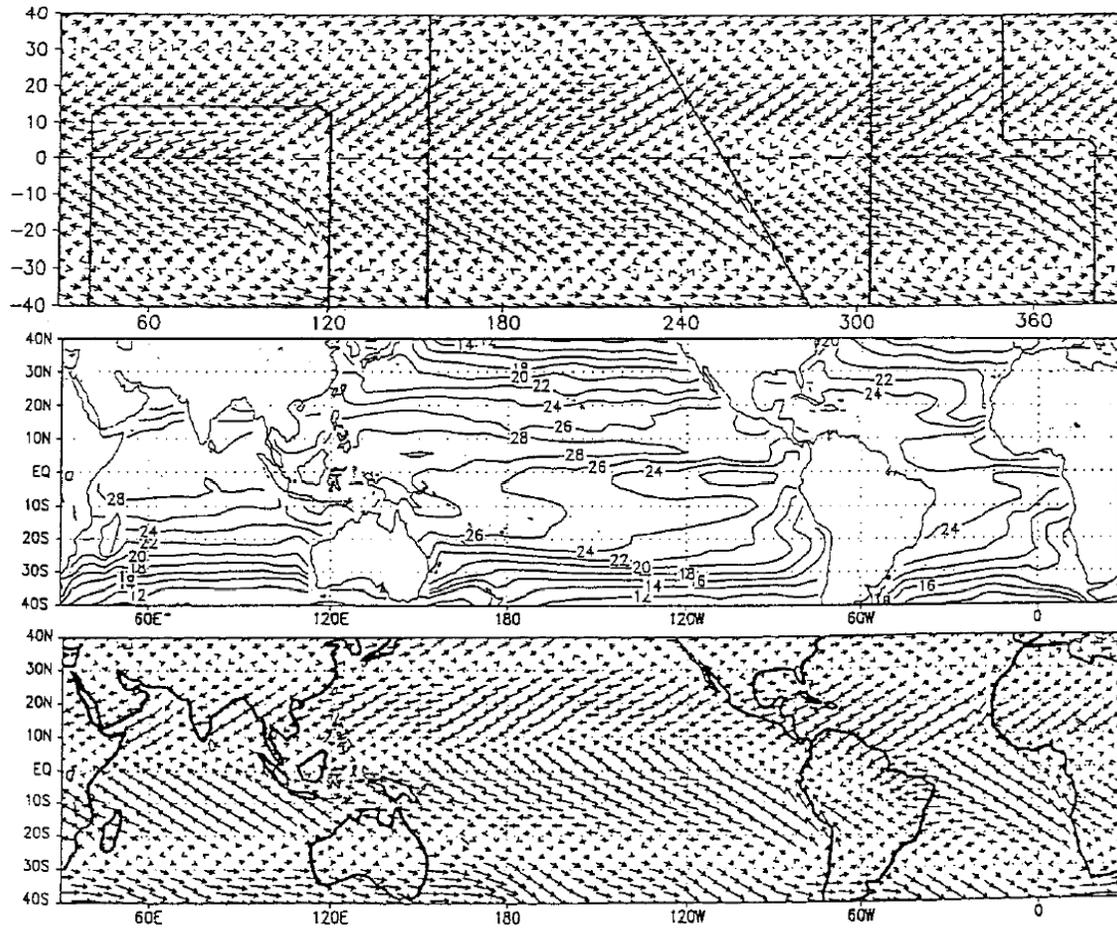
*Figure 4-8.* (top) Surface wind velocity in an atmospheric GCM forced with a specified SST distribution that is zonally uniform and equatorially symmetric. (middle) SST and (bottom) surface wind velocity in a coupled ocean-atmosphere GCM. The equinox insolation distribution is used and all the orography on land is removed. From Philander et al. (1996).
