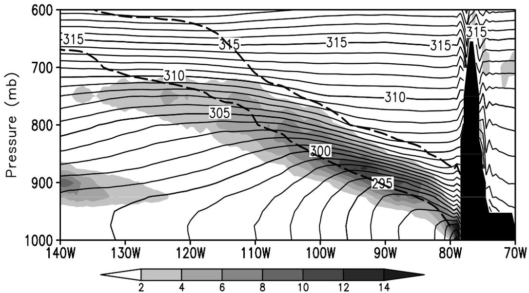
Figure 4-11. Simulated cloud liquid water content (shaded in  $10^{-2}$  g/kg) and virtual potential temperature (solid contours in K) in Xu et al.'s (2004) regional atmospheric model, averaged for August–October 1999 along  $10^{\circ}$ S. Dashed lines denote the boundaries of the inversion layer. The Andes are shaded in black.
