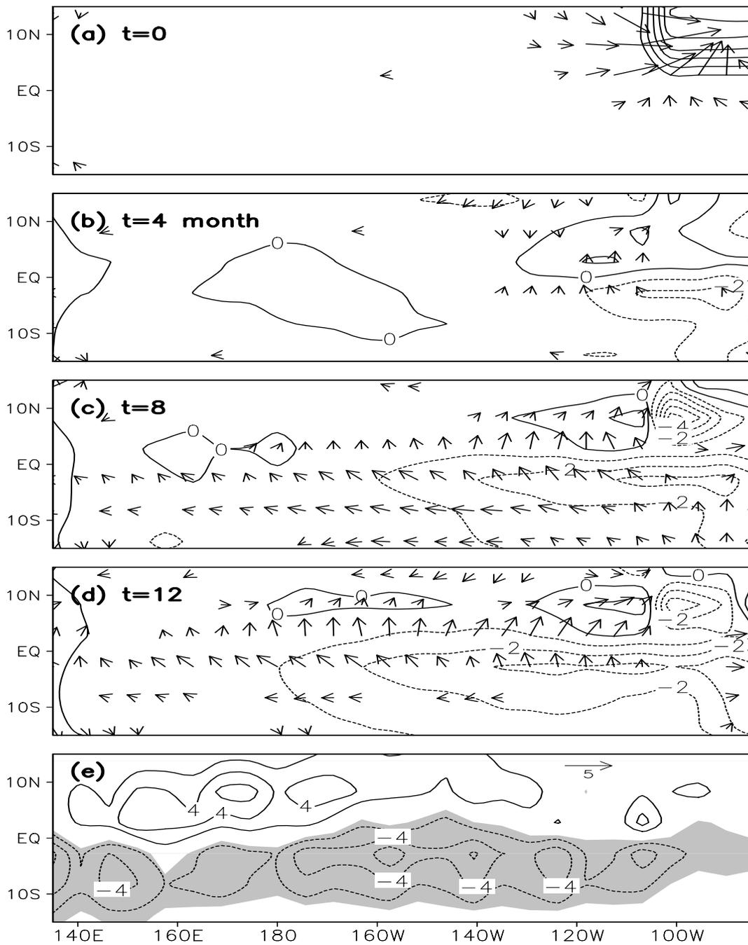
Figure 4-9. (a) Direct response of an atmospheric GCM to the addition of a northern land bulge: Anomalies of surface temperature (contours) and wind velocity. The evolution of surface temperature (contours in  $^{\circ}\text{C}$ ) and SST-induced surface wind velocity (m/s) changes 4, 8, and 12 months after the ocean model is turned on. (e) Changes in precipitation (mm/s) after the coupled model reaches a statistical steady state. From Xie and Saito (2001).
