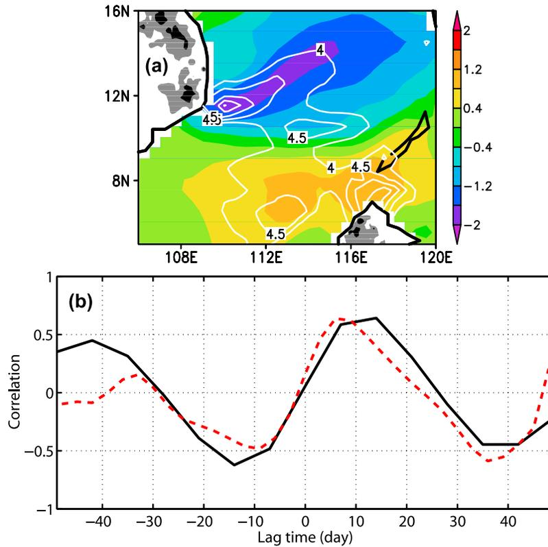
**Figure 9.** (a) EOF-1 of intraseasonal WSC (shaded areas), superimposed with standard deviation of intraseasonal Ekman pumping velocity (white contours, only the values  $>4 \times 10^{-6}$  m/s are shown here) during the same time. (b) Lead-lag correlation coefficients of PCs-1 between WSC and SSH (solid line is for observed SSH and dashed line is for OFES SSH). Land orographies greater than 0.5 and 1 km are plotted in Figure 9a with gray and black shading.
